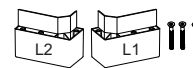
L - 700490 - Kit pé plástico (01x) L1 - Pés 70x100x50mm (03x) L2 - Pés 70x100x50mm (03x) L3 - Parafuso philips cabeça chata 3,5x40mm (18x) Foot / pie
